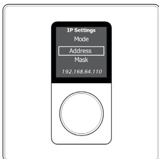
12. Tap the rotary encoder multiple times until the last digit of the IP address is selected.
