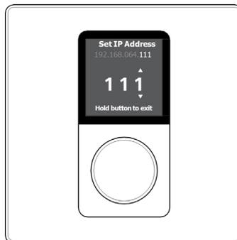
13. Twist the rotary encoder right (clockwise) to change the final digit of the IP address for this device – so it is not matching those of any other device also linked to the same amplifier. (e.g., for the second device change the final digit to #2; for the third device change the final digit to #3, and so forth).
